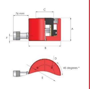
\*HLS101 features 2 base mounting holes at 90° from coupler
